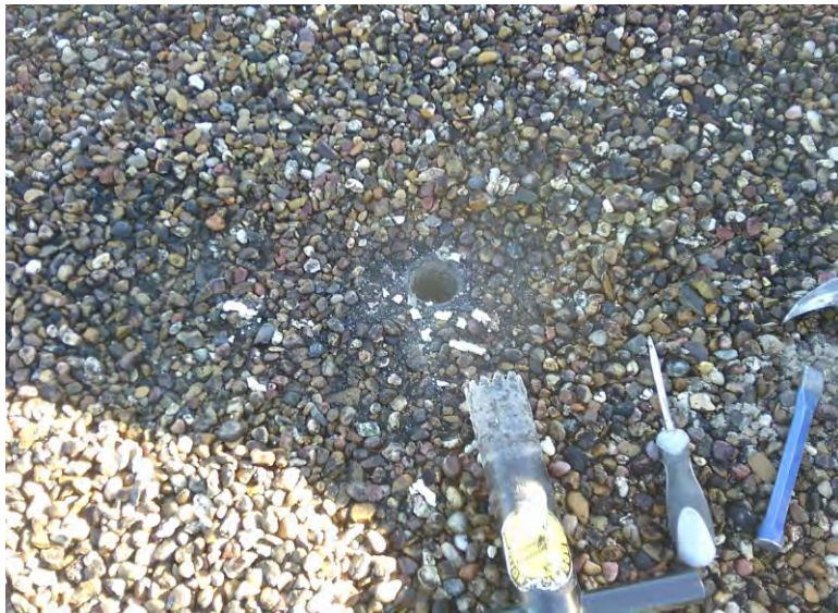
5. Asbestos Homogeneous Area 1 – Roof core materials / layers; Sample 01
